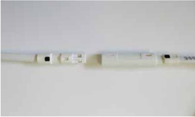
Male and female connectors fit together easily
